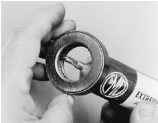
Figure 14: Applying lube to the thrust bearing
