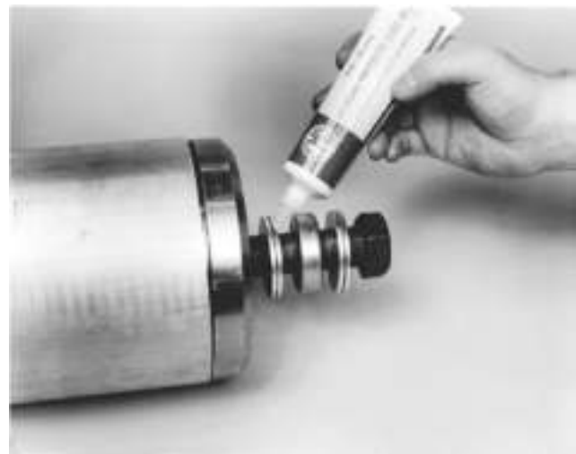
Figure 33: Apply lube to thrust washers
