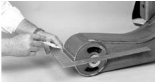
Figure 11: Marking bushing orientation on the bushing tube
