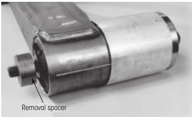
Figure 18: Installing removal spacer
