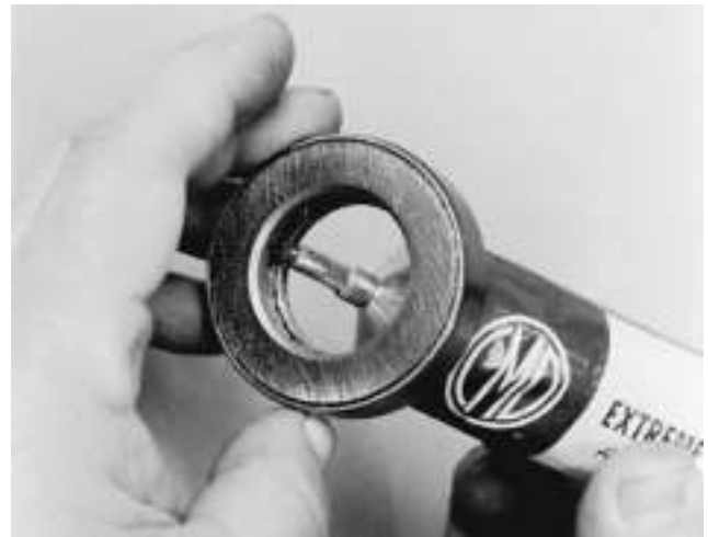
Figure 31: Applying lube to thrust bearing
