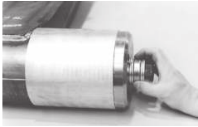
Figure 24: Ensure thrust bearing is free to turn
