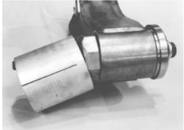
Figure 42: Continue to tighten hex head bolt after transition tube falls away
