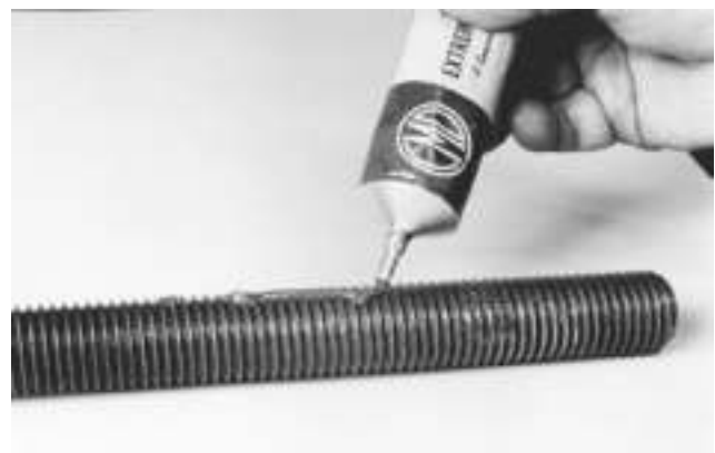
Figure 13: Applying lube to the hex head bolt
