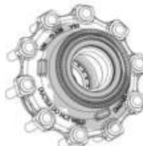
Figure 2: Check back side of hub for grease seal leak
